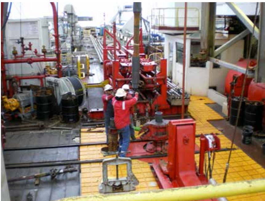
Removing a sediment core liner on board the RV JOIDES RESOLUTION during Expedition 320 of the Integrated Ocean Drilling Program (IODP).
