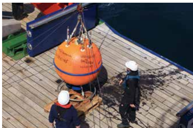
Recovery of a current meter moored in the ocean and installed in a flotation sphere. The current meters are deployed at different water depths for a year or longer and measure the current speeds and directions. These data provide evidence about fluctuations in the strength of ocean currents that is important for climate research.
