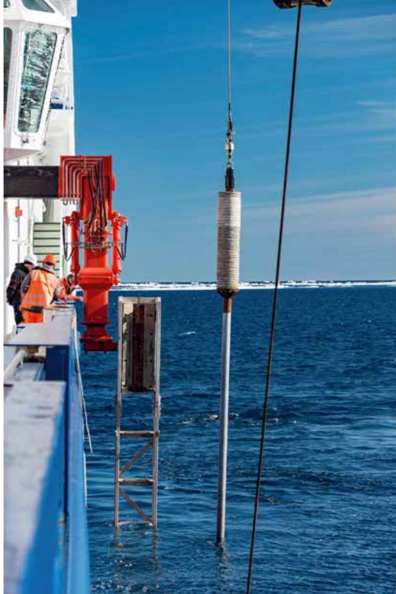
With a weight of several tons, a gravity corer can sample the seabed to a depth of about 20 meters.
